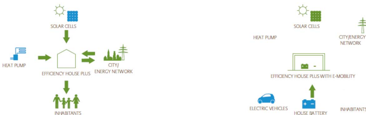
Figure 1: Schematic energy flows in the Efficiency House Plus with Electromobility [1]
